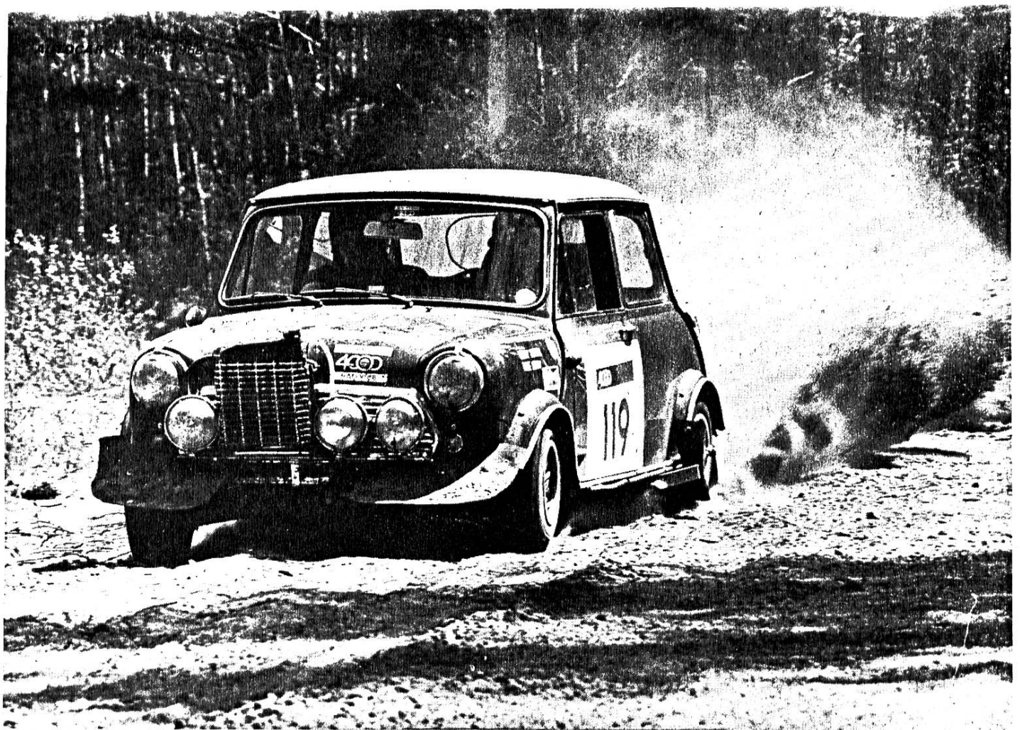
Optional extra? Overheating forced the BMC mechanics to fit the jury-rig radiator on the front of the Hopkirk-Kerry Cooper S; the car was disqualified for not complying to Group 2!
